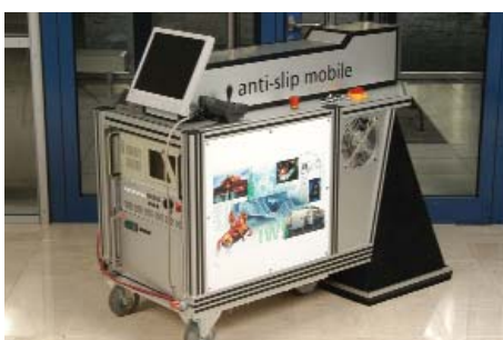
Mobile system for the anti-slip preparation of natural stones
