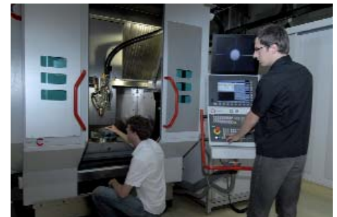
3 axes and 5 axes CNC milling machines with laser processing modules for the complete machining with laser buildup welding and milling
