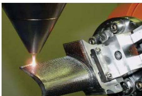
Repair of gas turbine blades through buildup welding with high power diode laser
