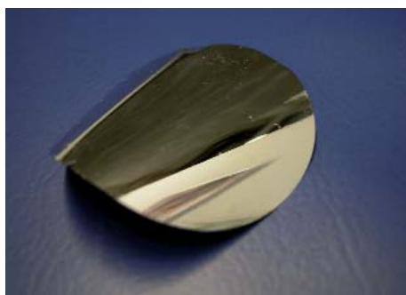
Fig. 3: Freestanding Ni/Al reactive multilayer coating, thickness 25 \mu\text{m} , diameter 50 mm
