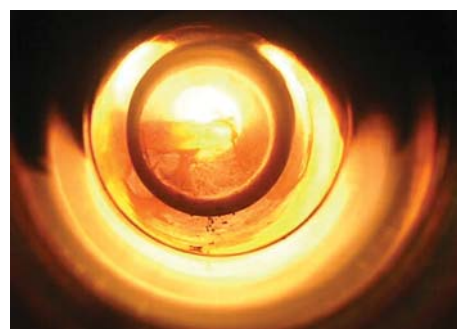
Arc synthesis of filaments made of carbon nanotubes
