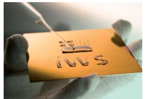
Hydrophilic / hydrophobic structured surface on a stainless steel sheet
