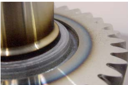
Fig. 3: Casehardened gear close to the weld seam
