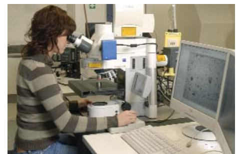
Laser scanning microscope LSM Pascal 5 for high precision characterization and analysis of surfaces in the micro and nano meter range
