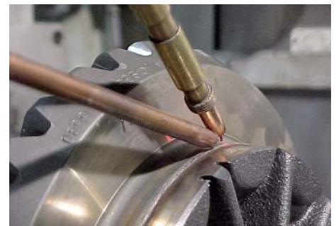
Fig. 7: Laser beam welding with filler material, differential transmission case (cast iron) with gear (casehardened steel)
