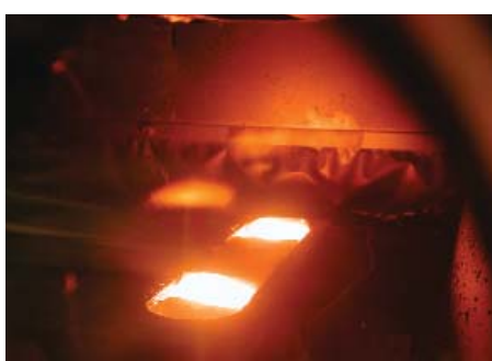
Metal evaporation through electron beam technology
