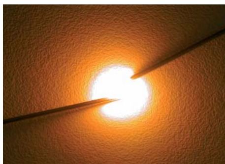
Fig. 2: Electrical ignition of a reactive multilayer coating
