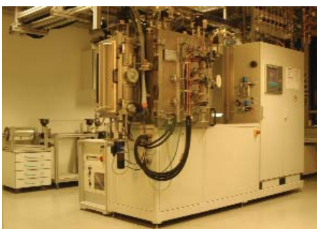
Equipment for the deposition of super hard amorphous diamond-like carbon coatings (Diamor®) based on the Laser-Arc process
