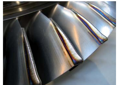
Fig. 2: Repaired edge geometry of a damaged blisk prior to the final finishing step
