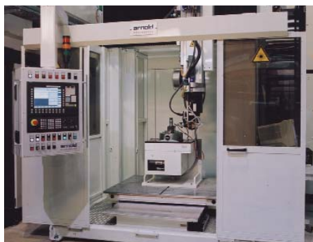
Laser beam welding system with 6 kW CO 2 high power laser
