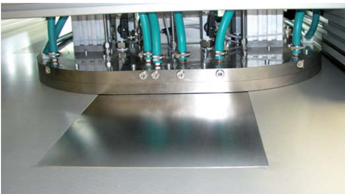
Fig. 2: Mobile AP-CVD processing head for the deposition on substrates of up to 300 \times 300\text{ mm}^2
