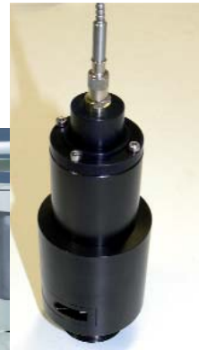
Brazing system of the company teamtechnik Maschinen und Anlagen GmbH Freiberg with an integrated temperature control system from Fraunhofer IWS, upper pic.: optics with filter holder
