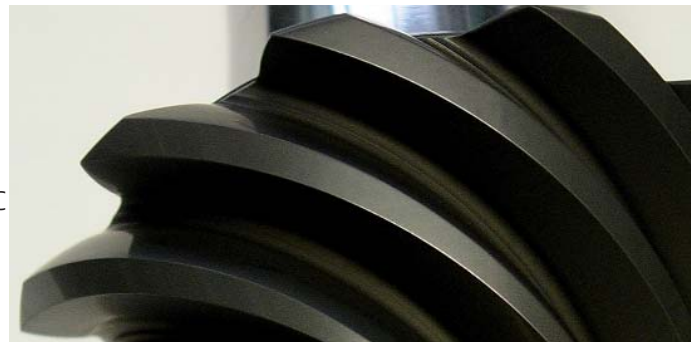
Fig. 3: A gear coated with an optimized ta-C/a-C multilayer coating
