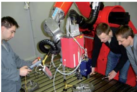
Installation of a robot based laser hardening system in Slovenia
