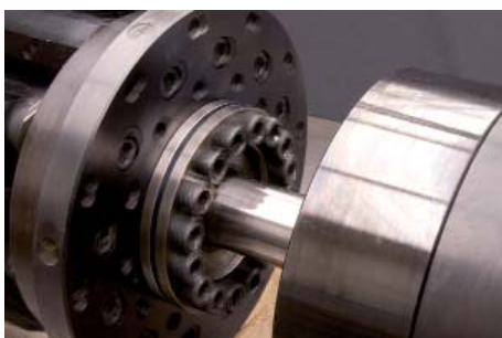
Servo hydraulic axial torsion test stand in action
