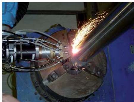
Laser beam buildup welding of ship components at Roussakis Ship Repairs in Greece
